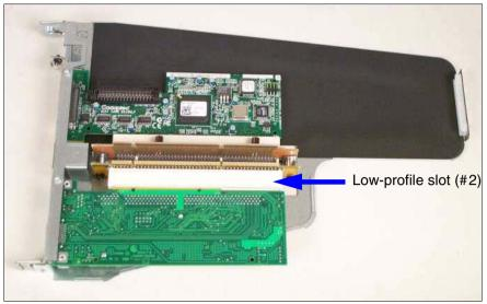
Figure 24: Installing the RSB S2 LP
